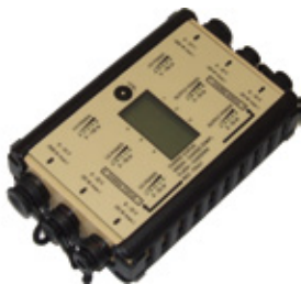
SFC POWER MANAGER, dimensions (LxWxH): 131 x 87 x 41 mm, weight: 0,48 kg
